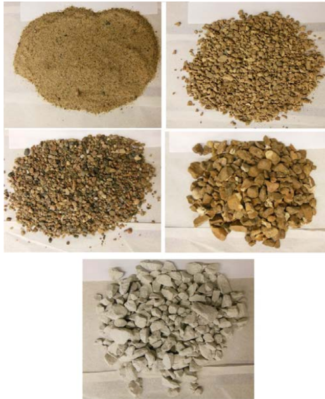
Figure 3.5. Aggregate types used in this study (one sand and four coarse aggregates)
