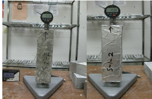
Figure 3.18. Shrinkage measurement of sealed (right) and unsealed specimens (left)
