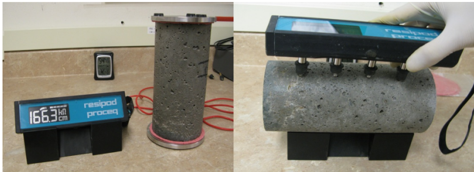
Figure 3.17. Bulk electrical conductivity (left) and surface resistivity (right)
