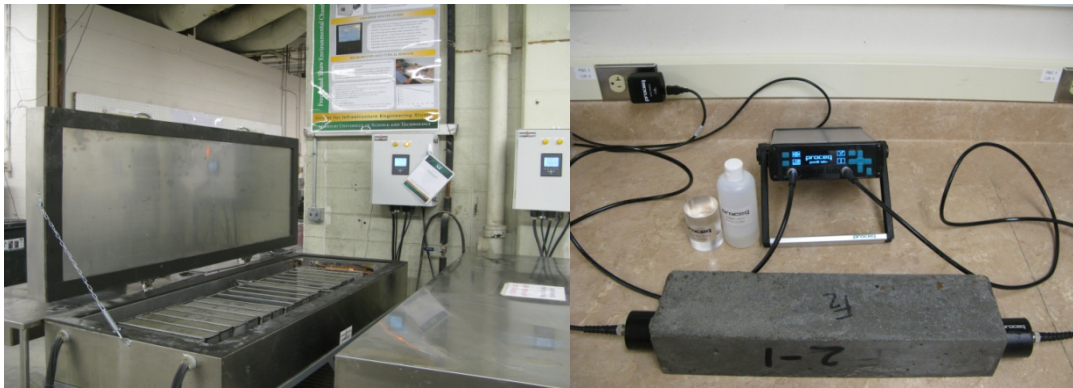
Figure 3.16. Freeze-thaw chamber (left) and ultrasonic velocity instrument (right)
