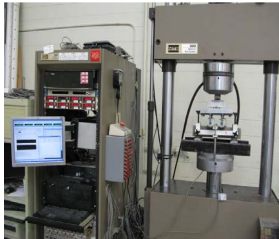
Figure 3.15. Test setup for flexural toughness measurement of FRC beams
