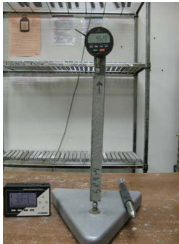
Figure 3.12. Measurement of free drying shrinkage
